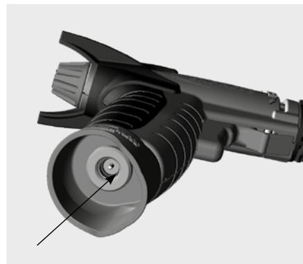
**1** Open the flow wheel to the maximum by turning in the direction of the + arrow and check the the lance is in the operating « position lightening bolt ».
